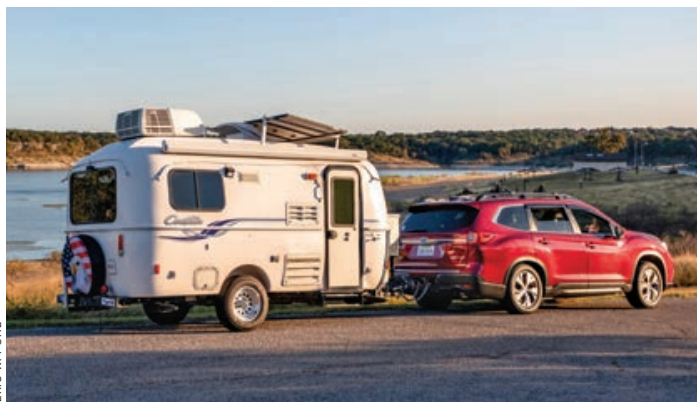
Studzinski’s compact camper includes rooftop solar panels and four 100-amp-hour batteries.
