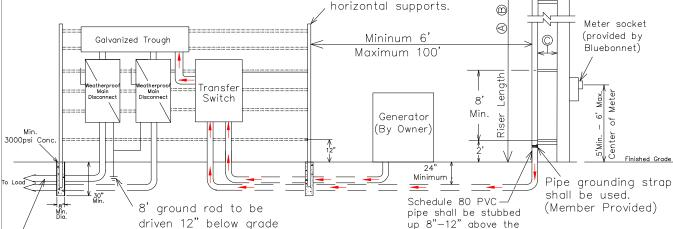
Service to load cable enclosed in minimum schedule 40 nonmetallic conduit.
