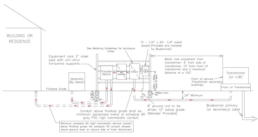
60-400 AMP 10 URD SERVICE TO A UNDERGROUND STANDBY GENERATOR SYSTEM WITH METER ON RACK OR BUILDING.
